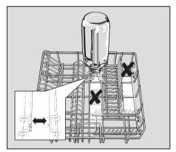
The bottle holder e.g. for milk or baby bottles, can be inserted into the bottom basket in more than one place. Position in any area marked white in the illustration. Do not position in areas marked "X", water cannot properly cover bottles in these areas.
